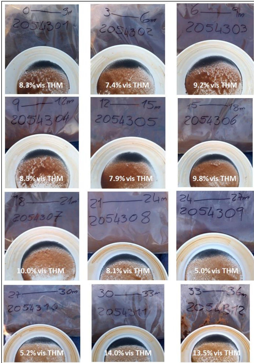
Figure 3: Field pan concentrate photos of samples from aircore drillhole 20CSAC543 showing the mineralised profile (beginning top left) and the high grade mineralisation discovered in the main Nhacutse zone.
